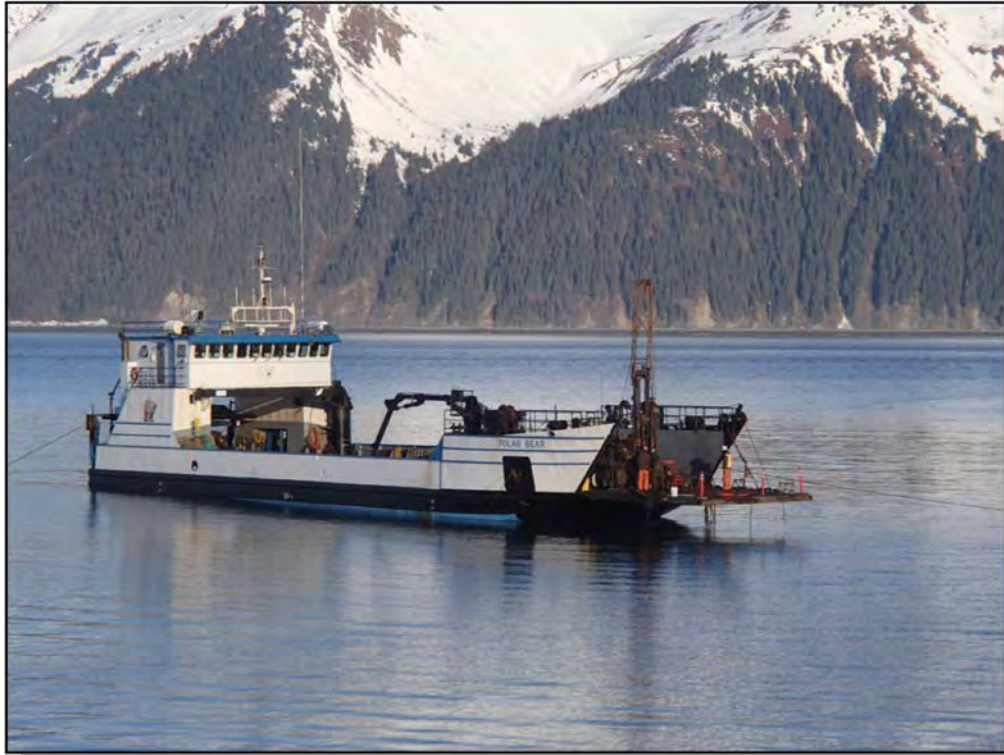
Photo 1: Landing craft with truck mounted drill-rig at rear of vessel (24 May 2013).
