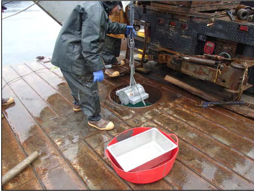
Photo 3: Obtaining surface sample from seafloor using Peterson Grab Sampler (24 May 2013).
